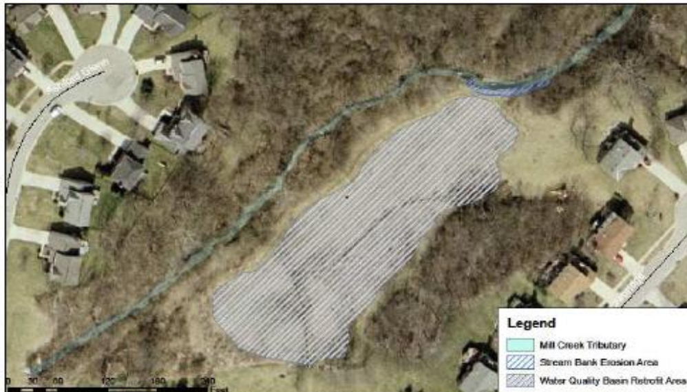
The streambank stabilization project protected the Beckett Water Quality Basin from an un-named Mill Creek tributary that was cutting into the basin's northern end. A heavy rainstorm in late June 2009 caused the stream to overflow onto the water quality basin, but the recently stabilized streambank held firm.
