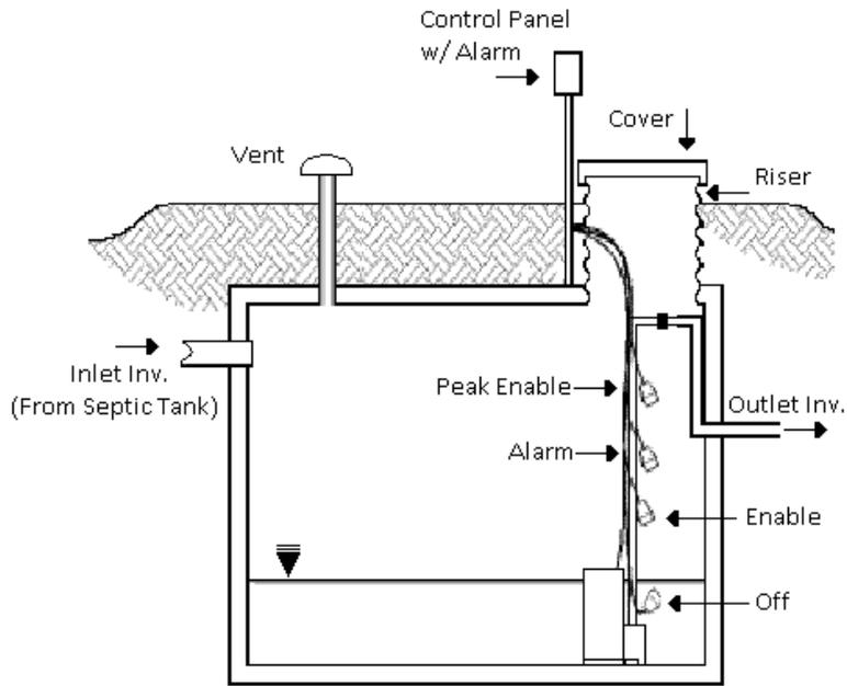
Note: The effective volume of the dosing chamber typically is based on the average daily flow and the filling time should not exceed 30 minutes unless flow equalization is provided.
