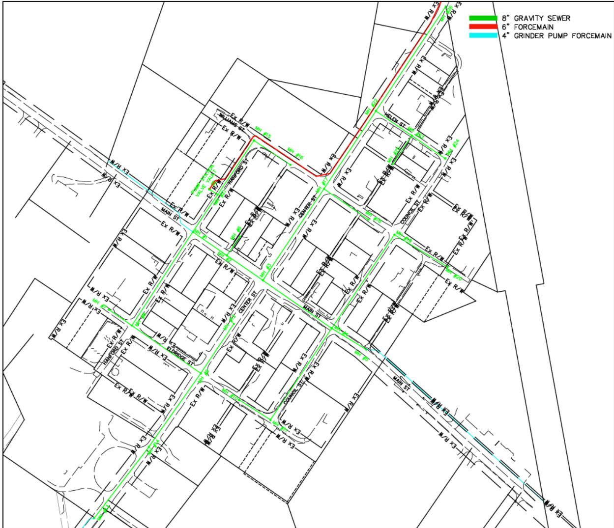
**Figure 4. Map of Lewistown collection system and new pump station located on the corner of Hanford Street.**
