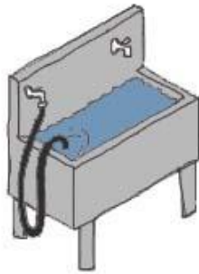
Example of a cross connection: hose in dirty water.
