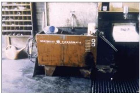
*DON'T handle waste or chemicals in areas where spills could enter a floor drain. This solvent parts washer is located right next to the floor drain.*
