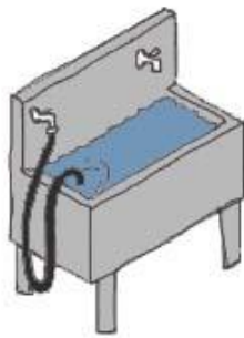
Example of a cross connection: hose in dirty water.
